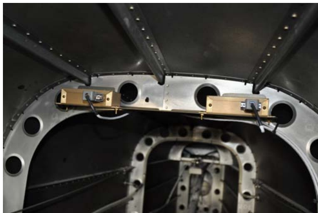
Magnetometer location in our RV-10 that has worked well.
